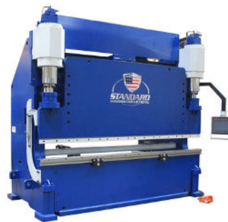
Y1-Y2 Model EV Precision Brakes (+,- .0004" ram repeatability)
